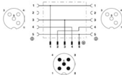
**M12 to M8 "Y" Splitter - Pin Out**
