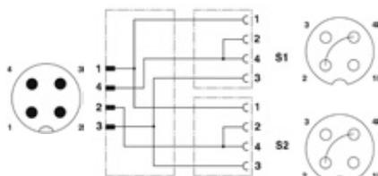
**M12 to M8 Cable Splitter - Pin Out**
