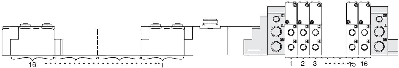
Shaded components are described by the assembly kit (AK) model number (see page 27). The communications module and number of I/O modules are described by the Electronic Interface (G3) model number designation (see page 27).
