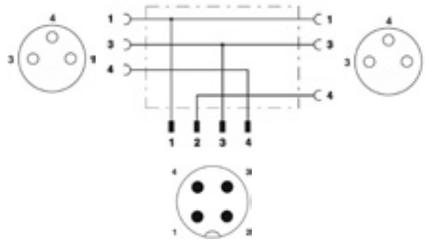
**M12 Field Wireable (IDC) - Pin Out**
